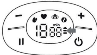
It takes approximately two hours to fully charge the Ardo Melia. As soon as three constantly lit bars are displayed during charging, the battery is fully charged. Now the pump has at least 100 min of expressing time. This duration may vary depending on the selected mode and vacuum level set.
