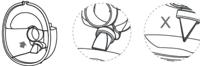
2. Insert the silicone diaphragm (c) into the collection cup (f) as shown and press down firmly.
