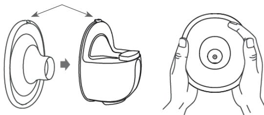
4. Fit the pump motor (b) as shown. Press firmly into place.
